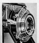
Synchro-switch (20) is set on the desired position (X or M). The distance, lens aperture, exposure time, and the shutter setting lever are set as
